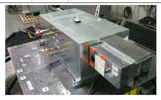
Unit was rigid base mounted to the shake table interface fixture four 1/2-inch diameter Grade 5 bolts, one on each corner of the unit, using the manufacturer-provided mounting tabs.
