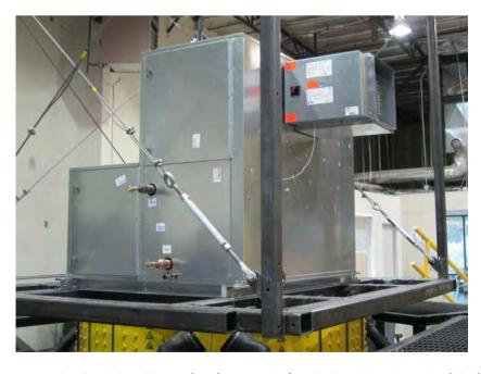
Unit was rigid base mounted to the shake table interface fixture with 1/2-inch threaded rod at each of the four corners.
